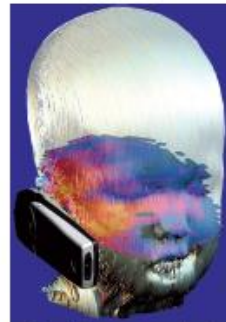
Computer simulation of the field distribution induced in the head tissues by a mobile phone
